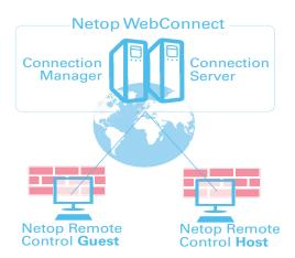
When you need to perform a remote control session the Guest sends a signal to the Connection Manager and a connection is established using WebConnect's Connection Server – an advanced router which manages and routes the traffic between Guest and Host.
