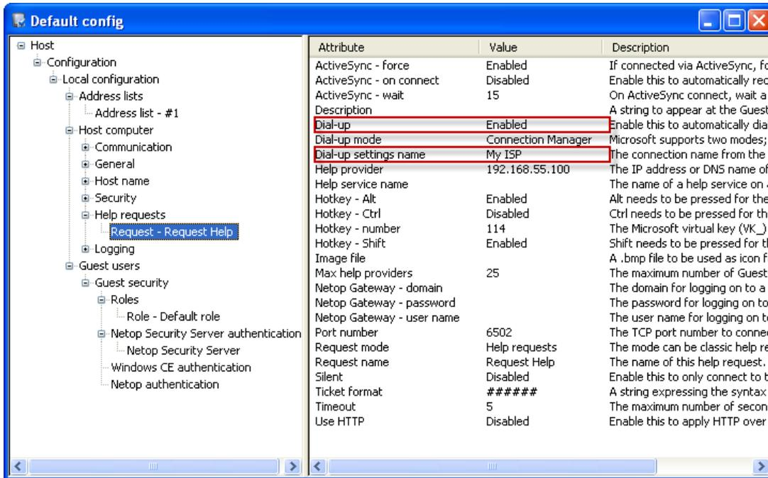
**Dial-up:** If enabled, Netop Mobile will establish a network connection through the Connection Manager when using the issuing of a Help Request. If disabled, dial-up will be prohibited.
